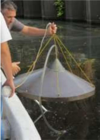
Person 1 is on the left and person 2 is on the right with the gas collection apparatus:
