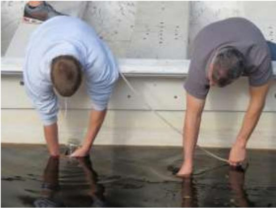
Person 1 screws the lid on the mason jar trapping the gas inside
